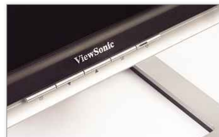
Make sure your faulty monitor's 'source' button isn't stuck or clogged with dirt
